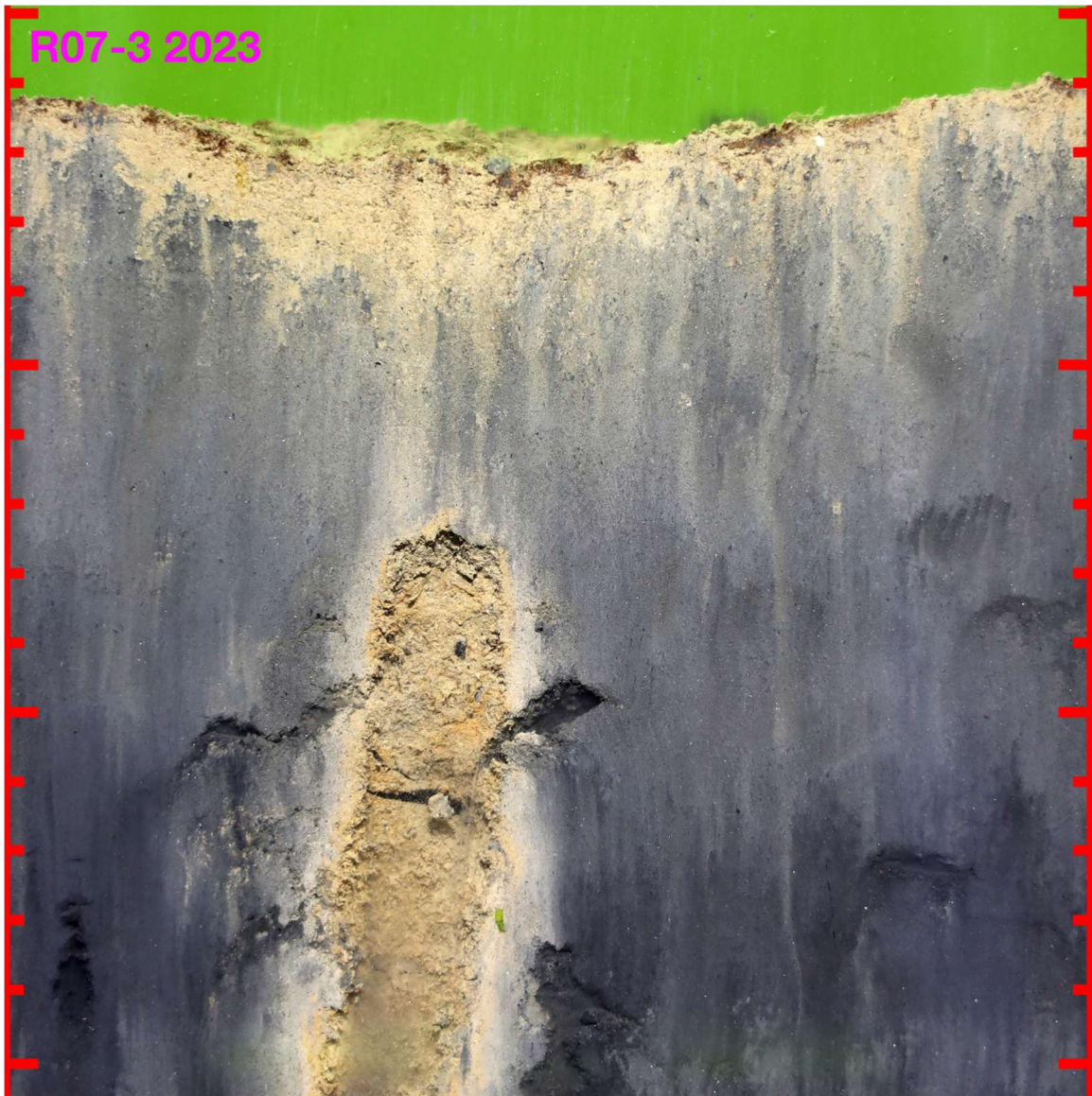
Figure 4-11. Example of a sediment-profile image, showing a large mantis shrimp burrow at Station R07, at Deer Island Flats, near the location of the former Boston Harbor effluent outfall. Scales at the sides of the image are in centimeters.
