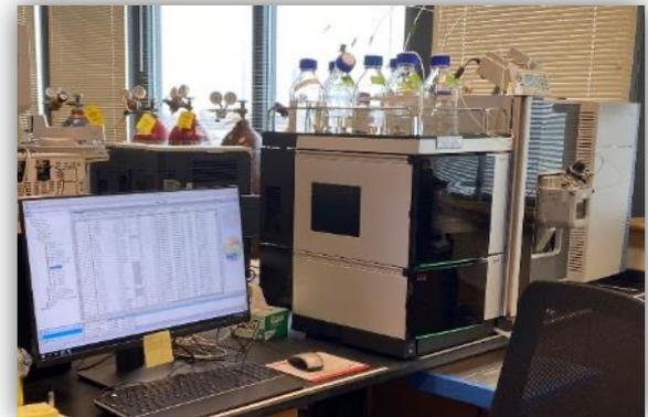
New lab equipment for analyzing PFAS in both drinking water and wastewater
