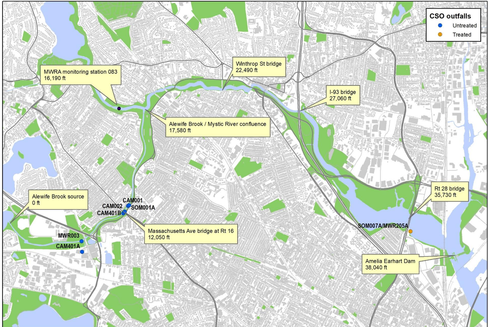
Figure 4-3. Alewife Brook/Upper Mystic River CSO Location Plan and Longitudinal Measurements from Alewife Brook Source (0 ft) to Amelia Earhart Dam (38,040 ft)
