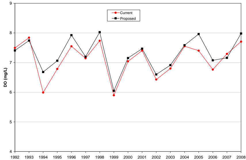
Figure 3-11 Bottom water dissolved oxygen annual minima for current (7 stations) and proposed (4 stations) survey designs.
