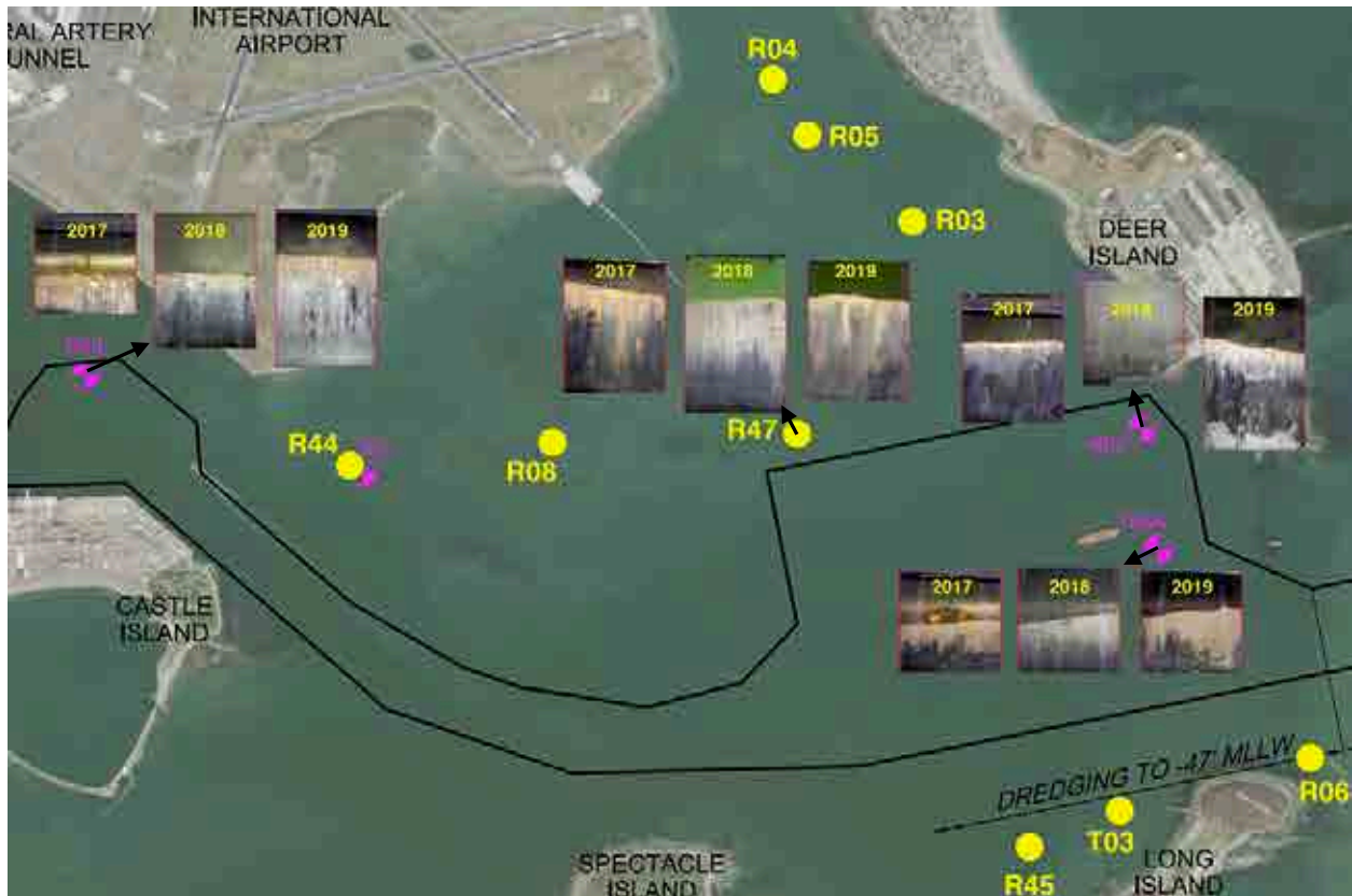
Figure 3-27. Changes at stations within the boundaries of President Roads dredging, part of the Boston Harbor deep draft navigation improvements. Black arrows from the station symbol to the 2018 image indicate the stations and their corresponding SPI images.
