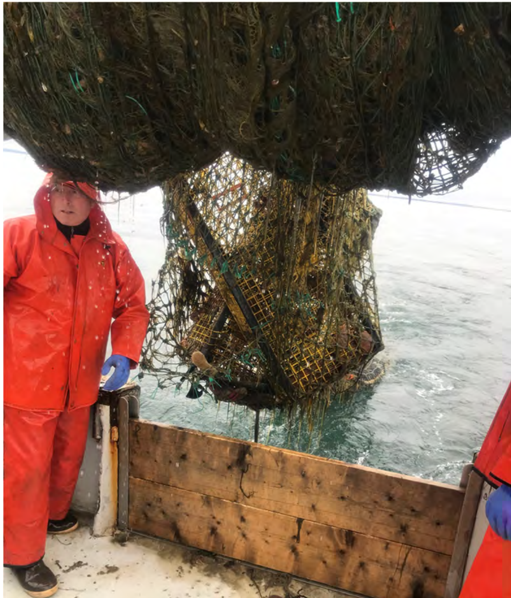
Figure 5-2. Lobster gear in flounder net trawl. Photo credit Michael Moore, Woods Hole Oceanographic Institution
