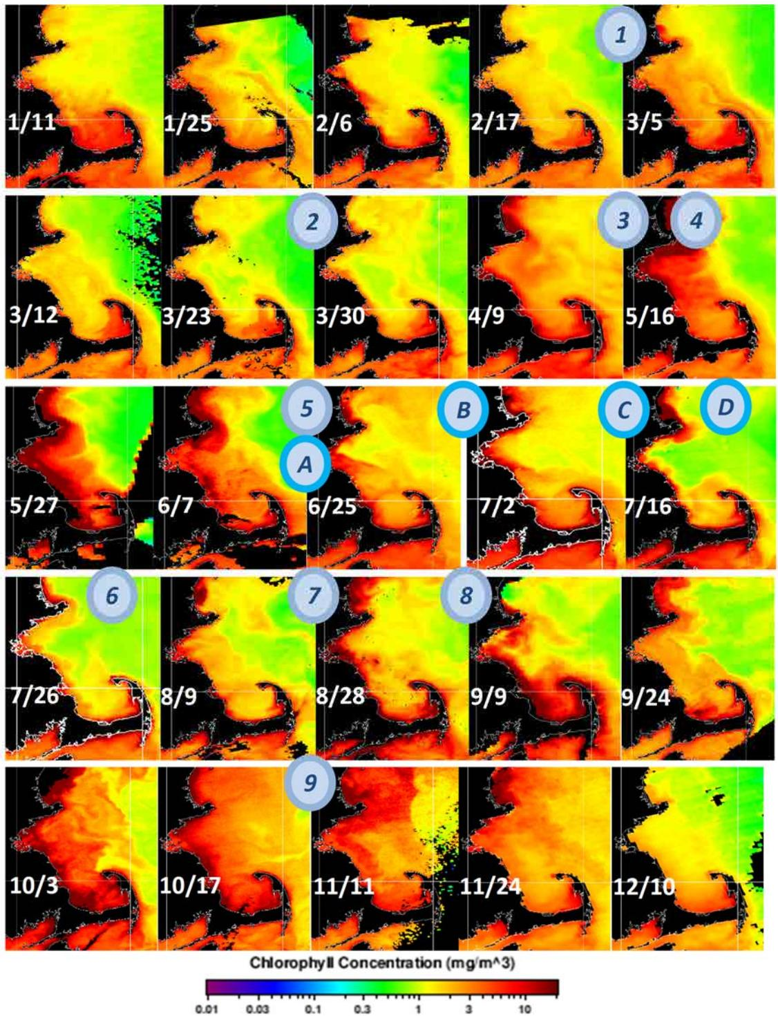
**Figure 3-8. Moderate Resolution Imaging Spectroradiometer satellite imagery of surface chlorophyll concentrations in 2017.** These images are heavily weather dependent and do not represent consistent intervals of time. The numbers and letters show the timing of the nine regular and four special MWRA surveys.
