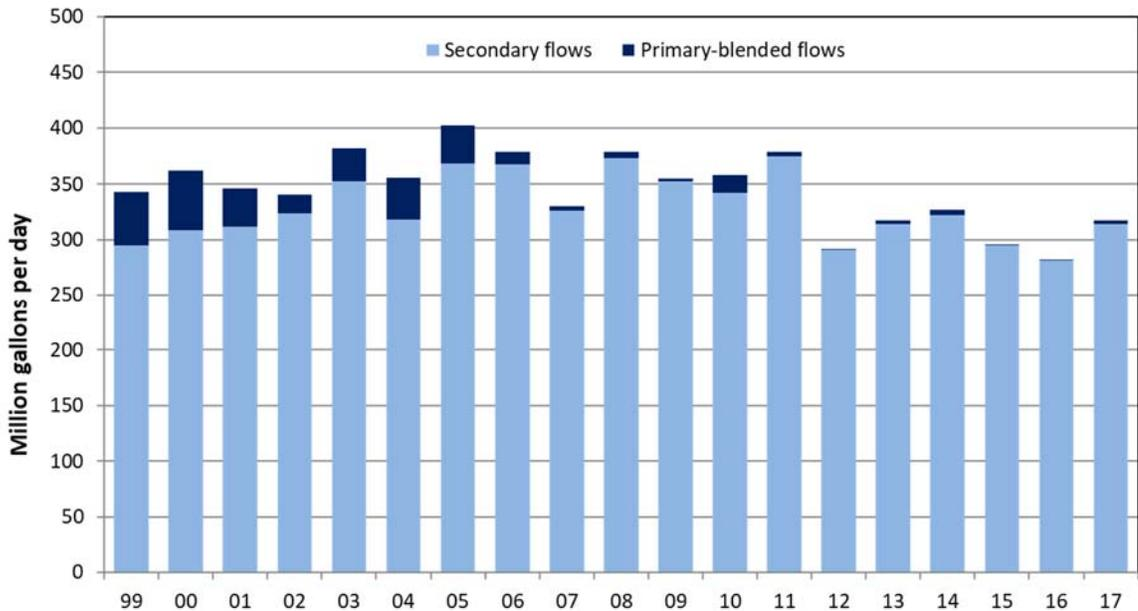
**Figure 2-2. Annual primary-blended and full secondary effluent flows, 1999–2017.** During large storms, flow exceeding the secondary capacity of the plant is diverted around the secondary process. Primary-treated flows are blended into secondary-treated flows before discharge.
