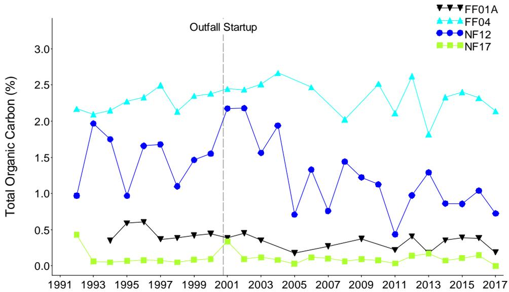
Figure 4-5. Total organic carbon at selected stations, 1992–2017. FF01A is the northern reference station; FF04 is within Stellwagen Basin; NF12 is >2km northwest of the outfall; NF17 is in close proximity and southwest of the outfall, where effects of the discharge might be expected.
