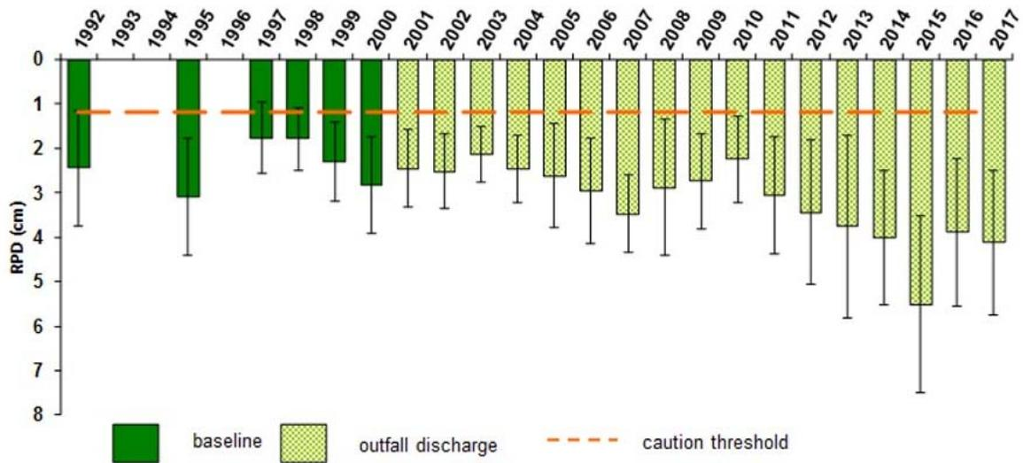
**Figure 4-9. Annual apparent color RPD depth for data from nearfield stations.** The mean RPD has been deeper than in baseline years, continuing to indicate that there has been no adverse effect from the discharge.
