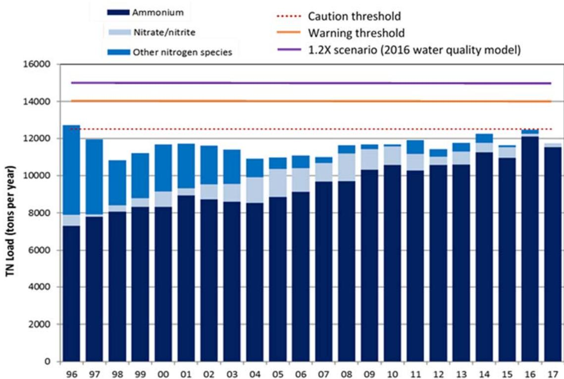
**Figure 2-5. Annual nitrogen loads, 1996–2017.** During outfall planning, managers and regulators assumed that discharges would total 14,000 tons per year by 2020. TN = total nitrogen, 1.2X scenario = a 20% increase over the actual 2016 load
