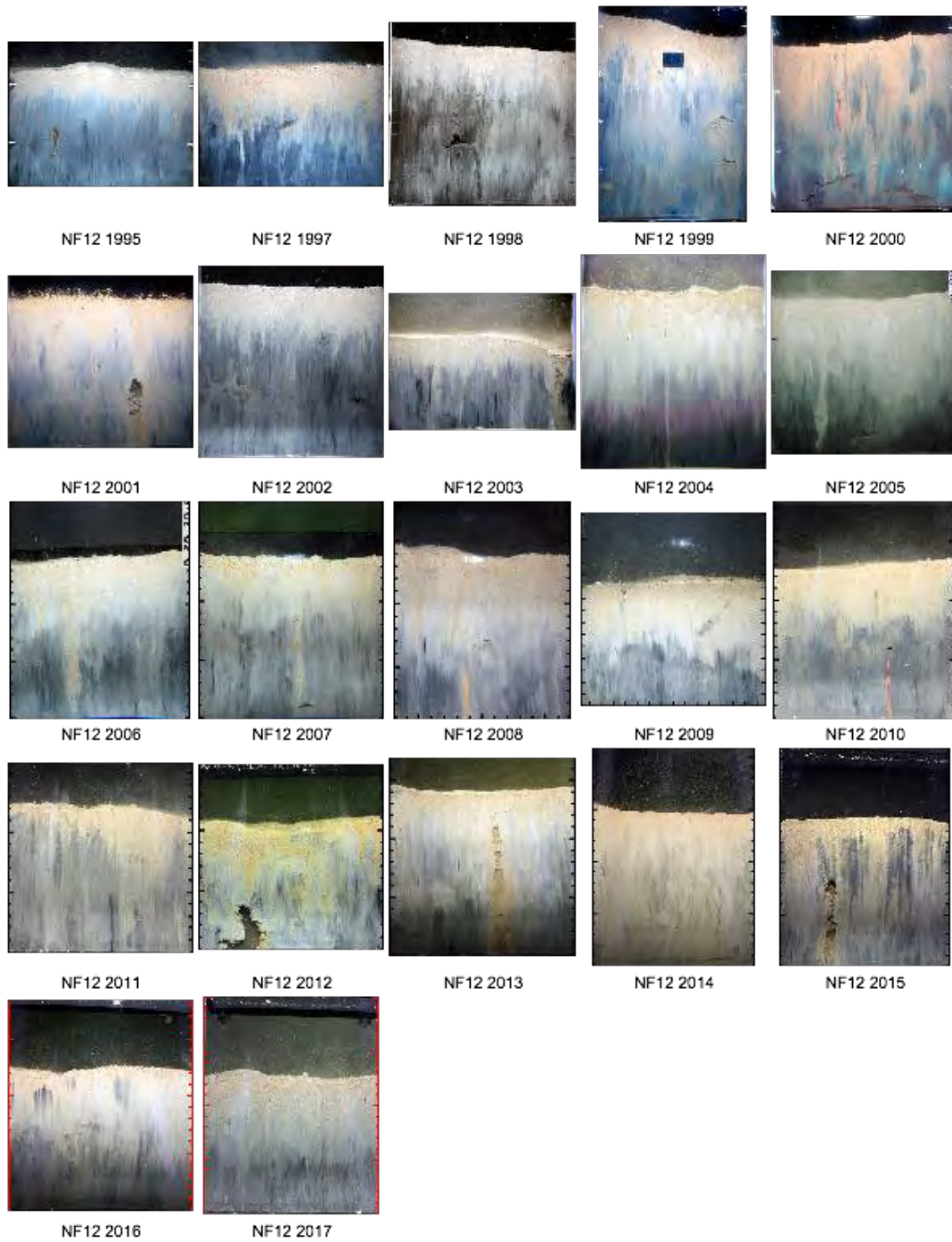
Figure 3-28. Mosaic of SPI images for station NF12 that had little temporal variation in grain-size. Scale on side of images is in cm.
