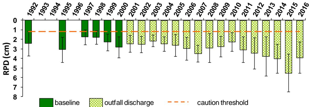
**Figure 4-7. Annual apparent color RPD depth for data from nearfield stations.** The average RPD discharge-period mean has been deeper than the baseline mean, continuing to indicate that there has been no adverse effect from the discharge.
