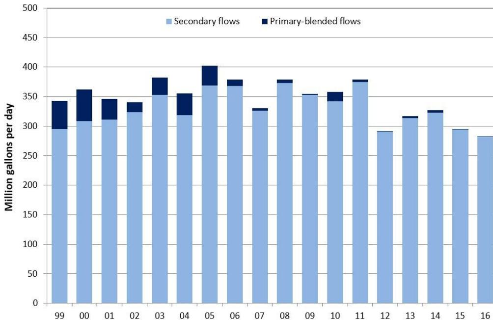
**Figure 2-2. Annual primary-blended and full secondary effluent flows, 1999–2016.** During large storms, flow exceeding the secondary capacity of the plant is diverted around the secondary process. Primary-treated flows are blended into secondary-treated flows before discharge.
