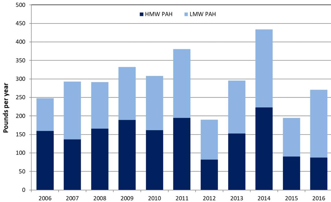
Figure 2-6. Annual polycyclic aromatic hydrocarbon (PAH) discharges, 2006–2016. LMW PAH = lower molecular weight PAH, HMW PAH = high molecular weight PAH
