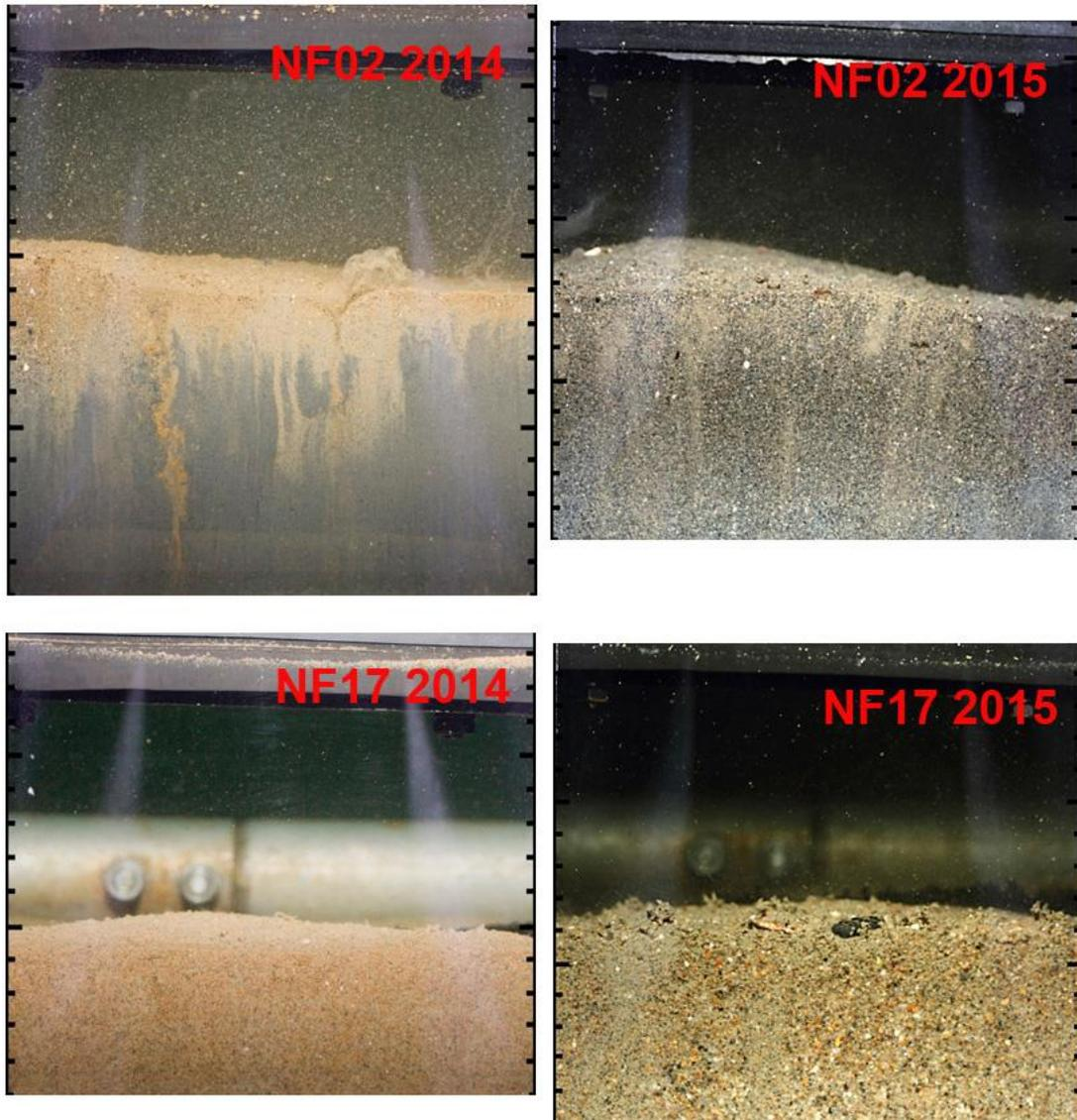
**Figure 4-7. Apparent change in sediment grain-size distribution between 2014 and 2015 at Stations NF02 and NF17.** Station NF02 is more than 5 km to the southwest of the outfall and changed from fine sand and silt to medium sand; NF17 is immediately to the southwest of the outfall and changed from fine-medium sand to medium sand.
