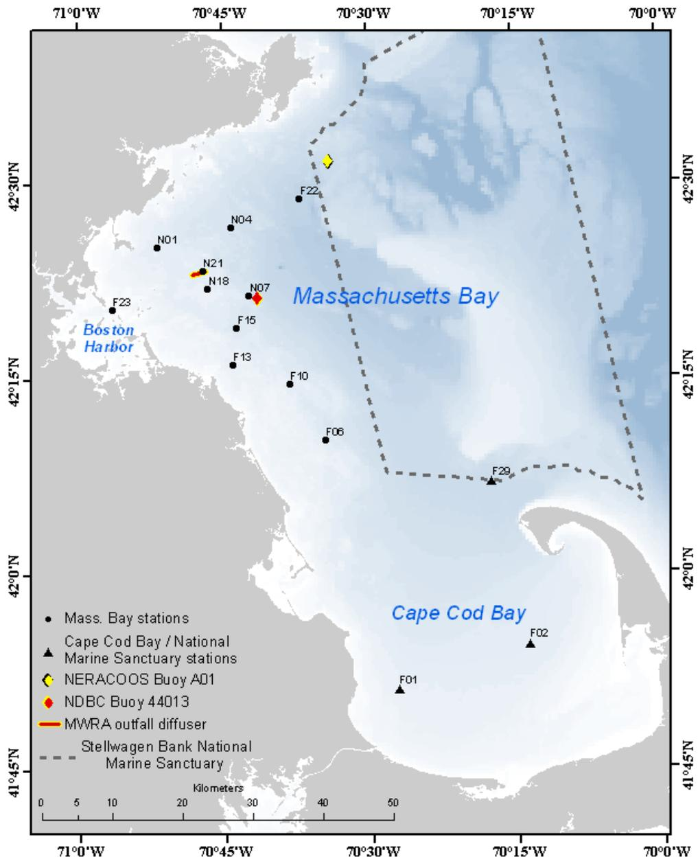
**Figure 3-1. Water-column monitoring stations.** Also shown are two instrumented buoys, one operated by the Northeastern Regional Association of Coastal and Ocean Observing Systems (NERACOOS) and the other by the National Data Buoy Center (NDBC); the MWRA outfall diffuser; and the Stellwagen Bank National Marine Sanctuary.
