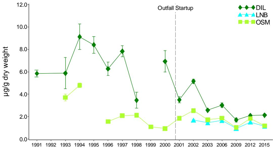
**Figure 5-7. Lead in deployed mussels, 1991–2015.** Gaps in data indicate years when concentrations in deployed mussels were lower than the pre-deployment controls. DIL = Deer Island Light, LNB = near the outfall, 1 kilometer south of the risers, OSM = Outfall Site
