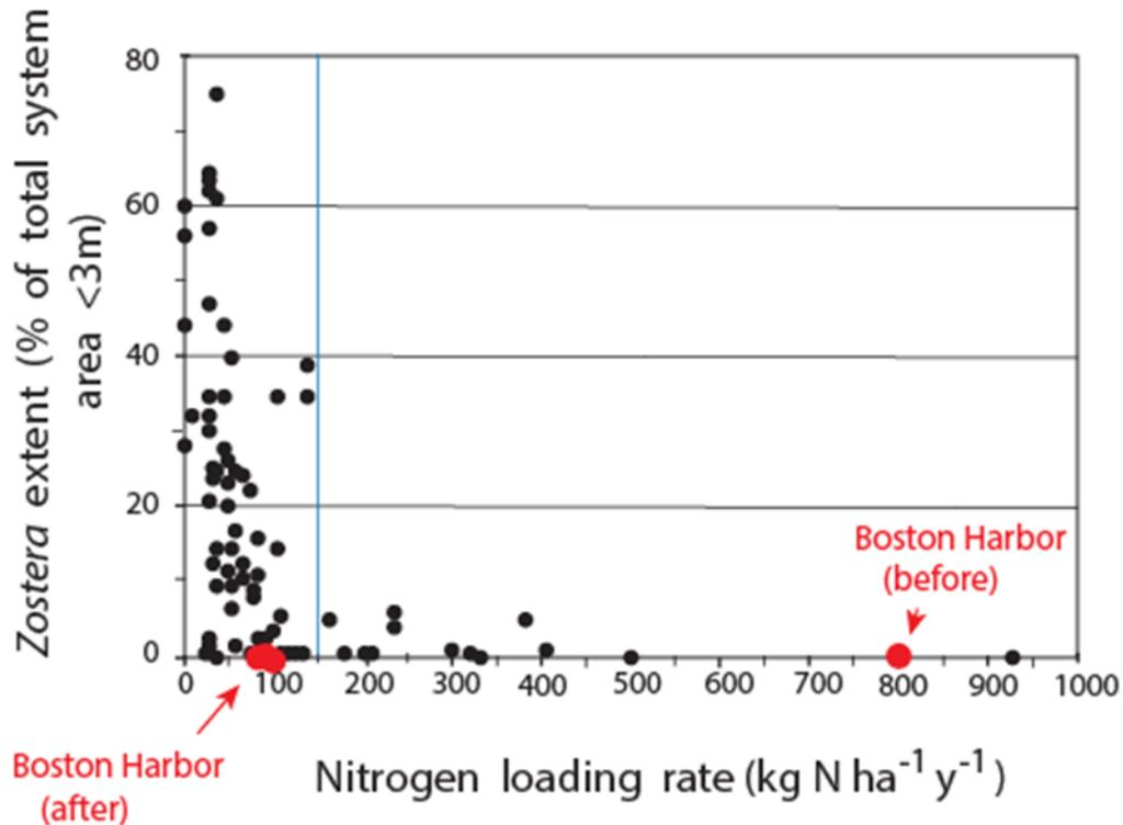
**Figure 6-1. Percent eelgrass coverage vs. nitrogen loading in coastal systems compared to Boston Harbor before and after the Boston Harbor Project.** The vertical blue line represents the 150 kg per hectare per year loading thought to allow for eelgrass beds in southern New England.
