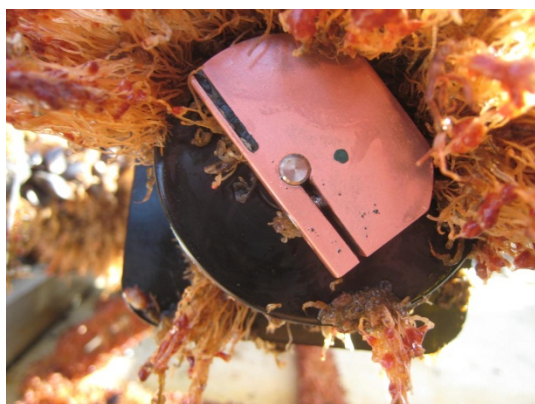
Figure 6. Example of extreme frondular biofouling by colonial hydroid polyps on the ECO FLNTU observed upon recovery of deployment 30. Photo credit M. Mickelson.
