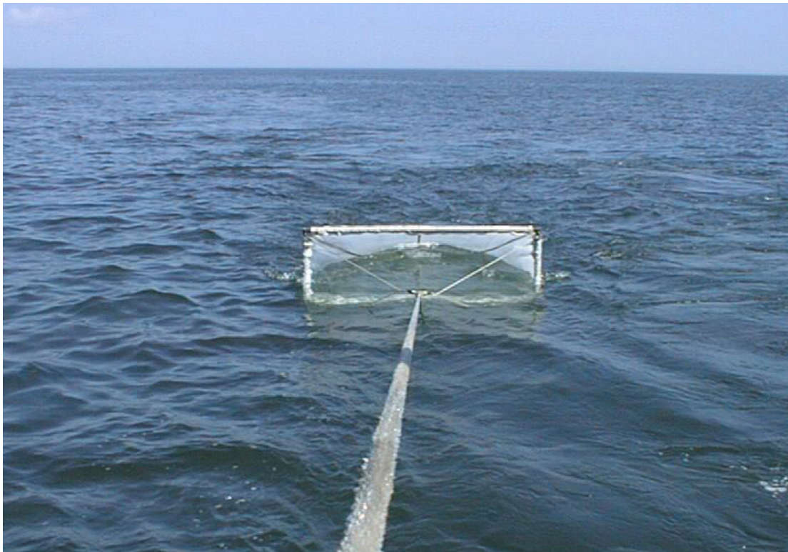
Figure 6-1. Net used for sampling floatable marine debris. The net measures 1 x 2 meters, with 500- \mu m mesh.
