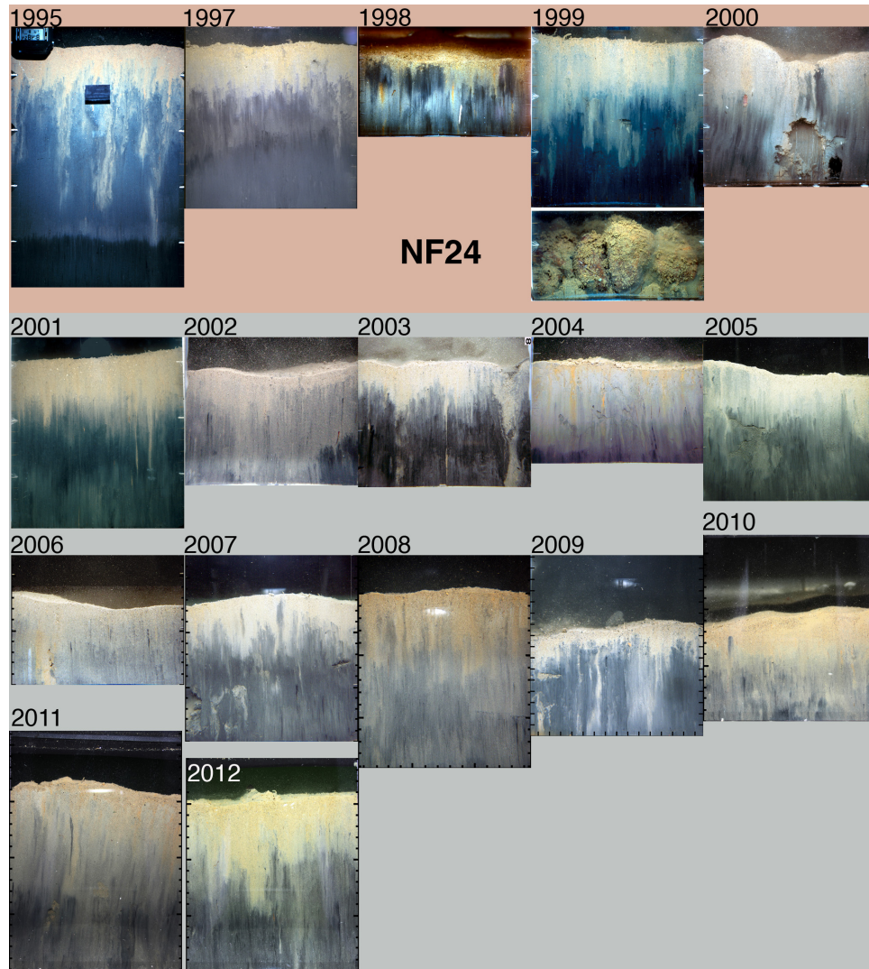
Figure 4-8. Thumbnail images from Station NF24, located within two kilometers of the outfall. There are no indications of increased organic carbon content or other outfall effects. Black hash marks are at five-centimeter intervals in images made prior to 2006 (many are quite faint). Hash marks in recent images are at one-centimeter intervals.
