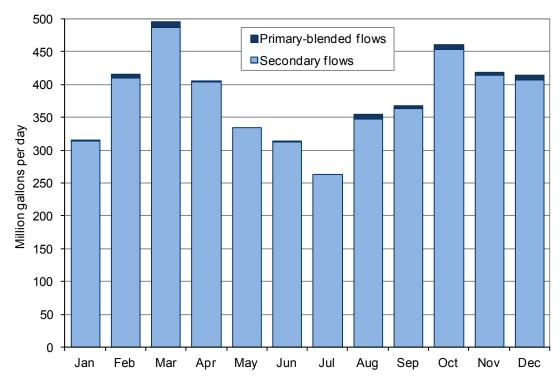
**Figure 2-2. MWRA primary-blended and full secondary effluent flows during 2011.** Amounts of blended flow were low in every month, despite the relatively wet year.
