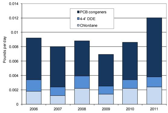
**Figure 2-8. PCBs and pesticides in Deer Island Treatment Plant discharges.** New methods were implemented in 2006 to detect these compounds, which are present at very low levels. (4-4' DDE is a breakdown product of the pesticide DDT. PCBs, DDT, and the pesticide chlordane were banned in the 1970s and 1980s but they persist in the environment.)
