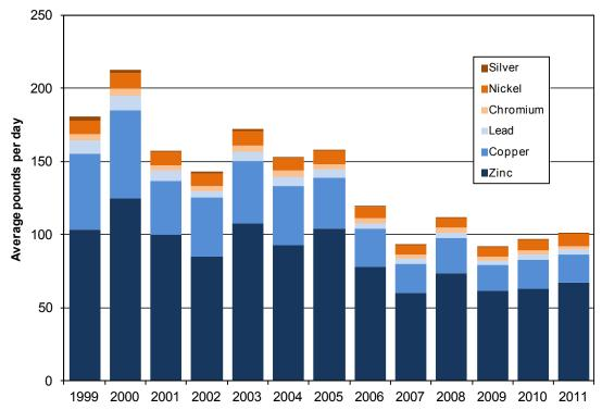
**Figure 2-6. Deer Island Treatment Plant metals discharges.** Except for copper, the metals meet receiving water quality criteria in the effluent, even without the dilution provided by the outfall.
