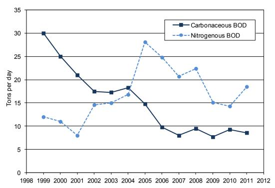
**Figure 2-4. Biochemical oxygen demand in MWRA discharges.** MWRA's permit limits carbonaceous BOD, which remained low in 2011. Nitrogenous BOD is the result of microbiological breakdown that occurs as a result of secondary treatment.
