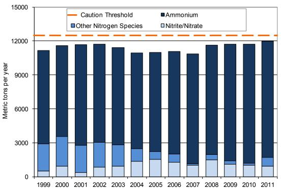
Figure 2-5. Deer Island Treatment Plant nitrogen discharges. Most of the nitrogen in the effluent is in the form of ammonium.
