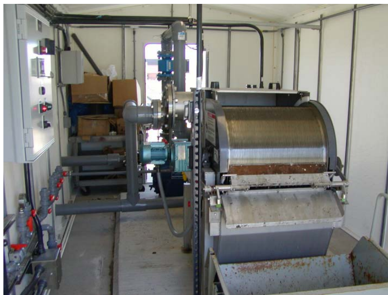
Figure 1. Effluent floatables sampling device
