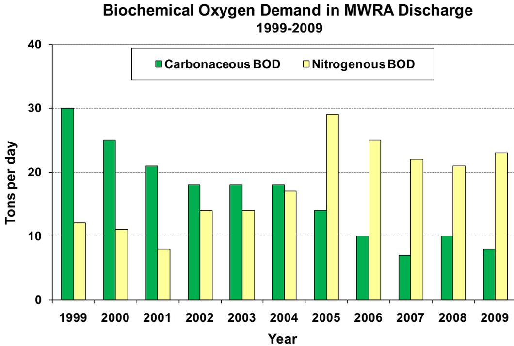
Figure 2-3. Biochemical oxygen demand in MWRA discharge. MWRA’s permit limits carbonaceous BOD, which remained low in 2009. Nitrogenous BOD is the result of microbiological breakdown that occurs as a result of secondary treatment.
