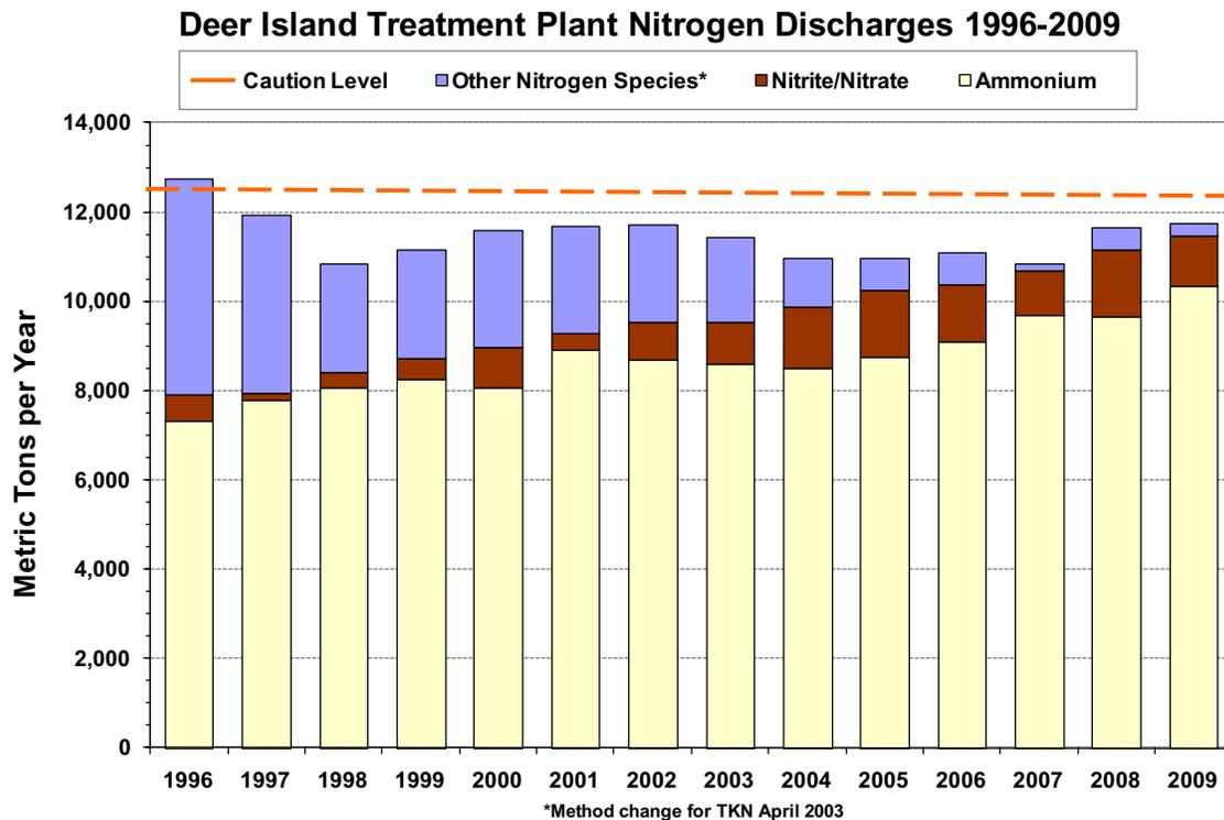
**Figure 2-4. Deer Island Treatment Plant nitrogen discharges.** Discharges of ammonium remained relatively high, a result of the secondary treatment process. (TKN = total Kjeldahl nitrogen, a measure of total nitrogen in the effluent)
