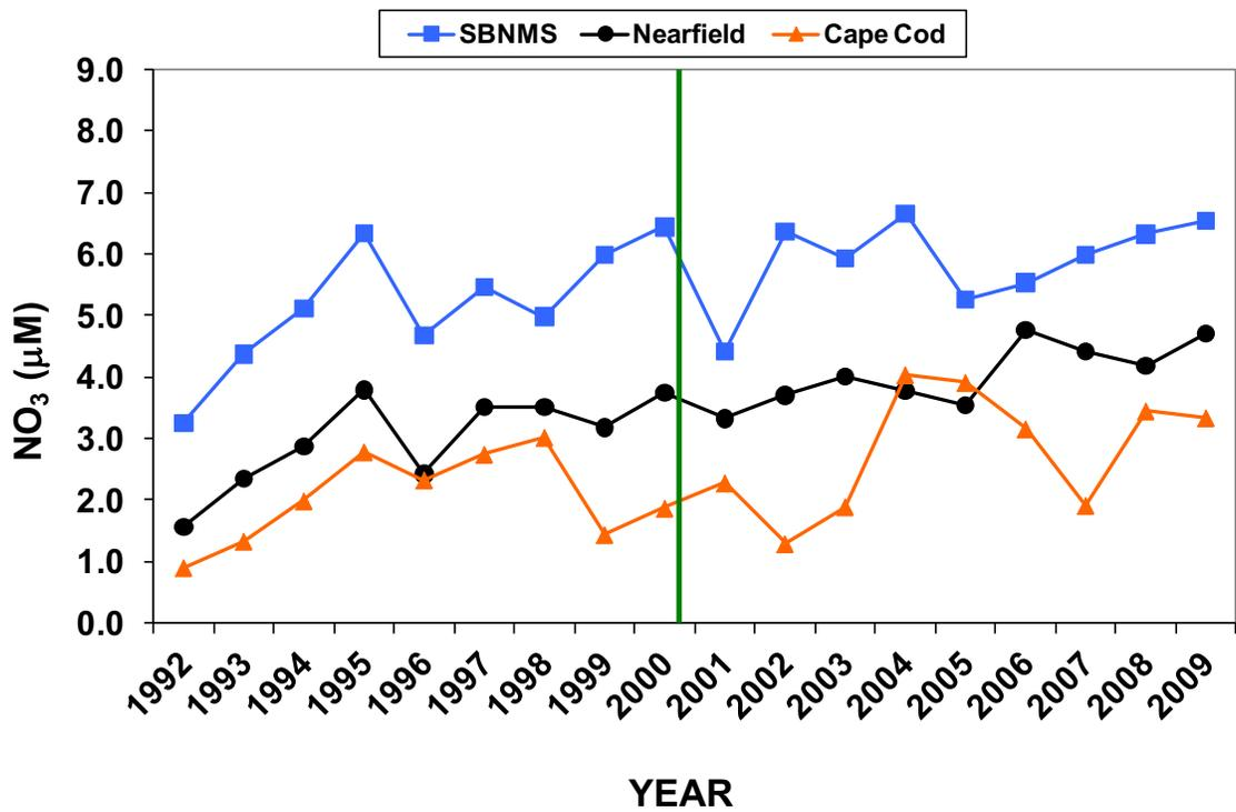
**Figure 7-5. Annual mean nitrate at the Stellwagen Bank National Marine Sanctuary (SBNMS), the outfall nearfield, and Cape Cod Bay.** Nitrate concentrations are variable, but there have been no changes that can be attributed to the outfall. Vertical line indicates when outfall came on-line.
