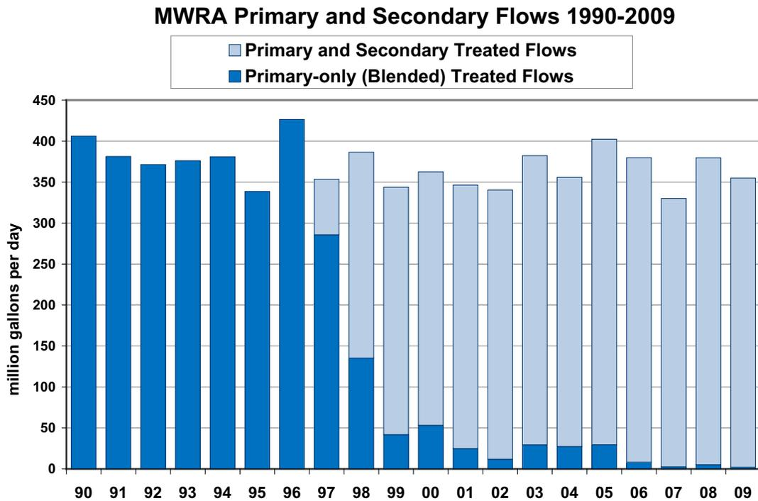
**Figure 2-1. MWRA primary and secondary effluent flows.** Almost all the flow from the treatment plant received primary and secondary treatment. (Primary-only flows are blended with secondary flows, and the blended flows meet permit limits.)
