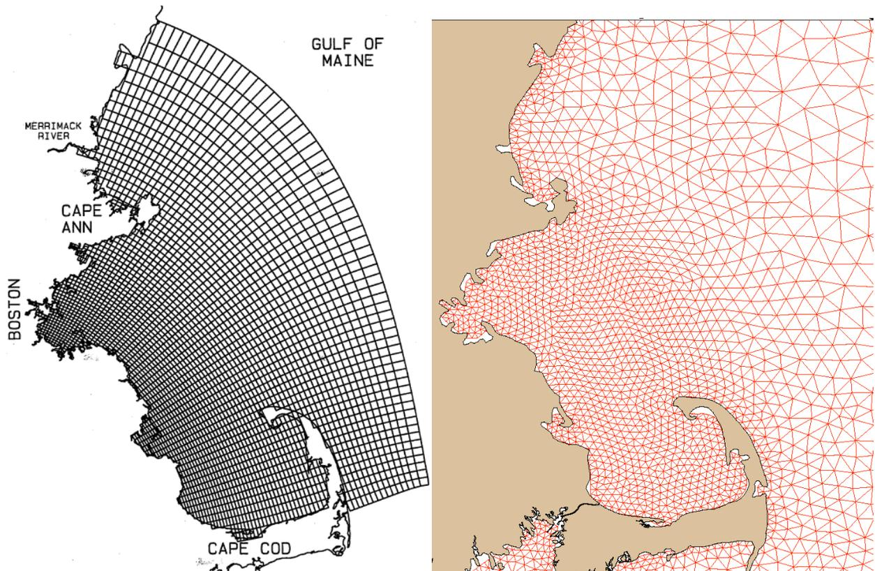
**Figure 6-1.** The BEM was initially based on a structured grid (left), but has been replaced by an unstructured grid, finite volume model (right), which provides a more accurate fit to the irregular geometry of the coast.
