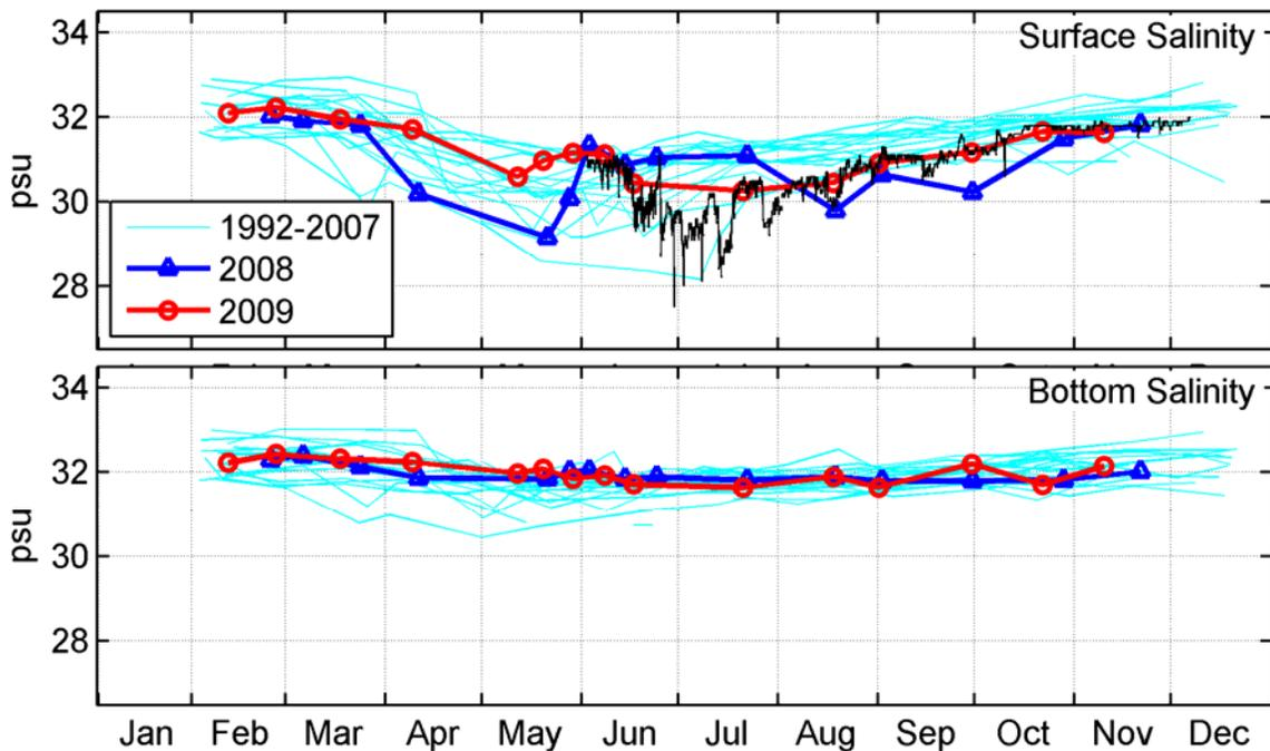
**Figure 2-8.** Comparison of the 2009 surface and bottom salinity near the outfall site (nearfield stations N16, N18 and N20) for 2009 (red line) compared to 2008 (dark blue line) and the previous 16 years of observations (1992-2007; light blue). The surface salinity data (June-December 2009) recorded at NOAA NDBC Buoy 44013 is in black.
