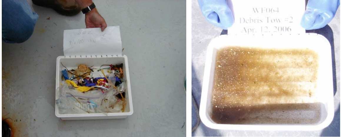
Figure 6-4. Samples of marine debris tows at the outfall site. On the left, a sample collected before the outfall went on-line has plastic marine debris. The picture on the right, collected after the outfall went on-line, shows the fat particles which are sometimes seen.
