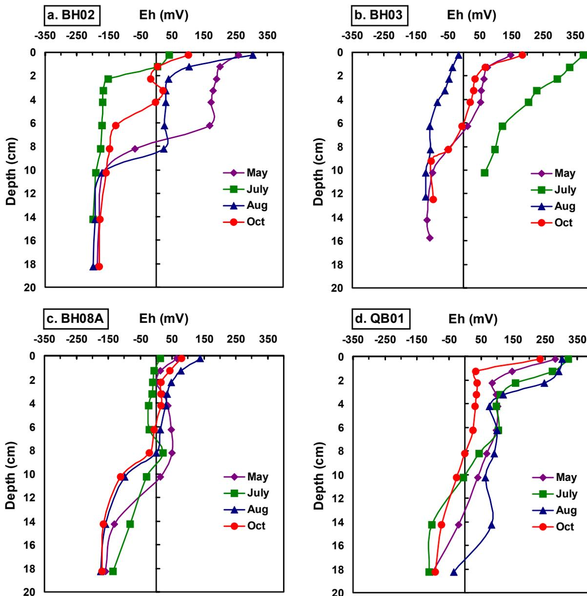
Figure 22. Eh profiles for May through October, 2003, from Harbor stations a.) BH02, b.)BH03, c.) BH08A, and d.) QB01.
