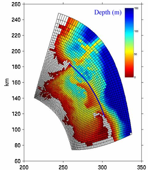
Figure 2.1. The model grids and bathymetry. The blue solid line in the figure indicates the BEM model domain.
