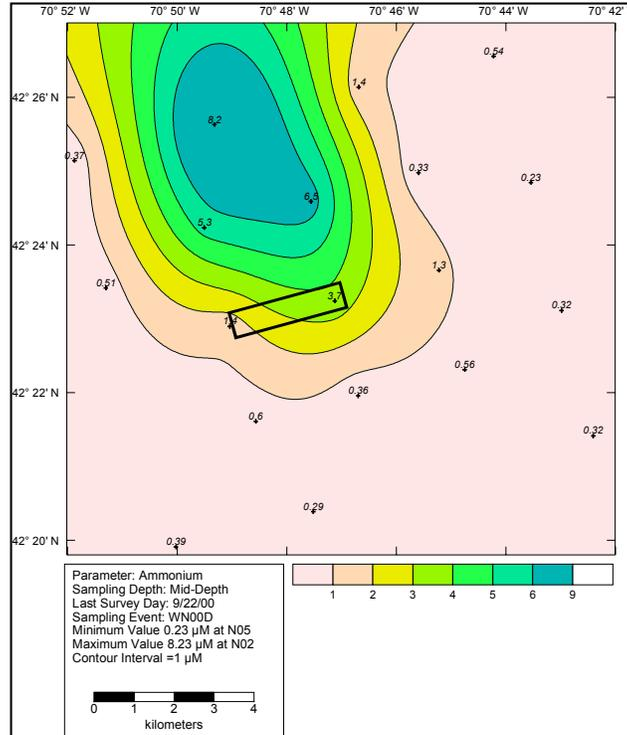
Figure 6-2. Horizontal contour of  $\text{NH}_4$  at the pycnocline. The rectangle represents the location of the diffuser.
