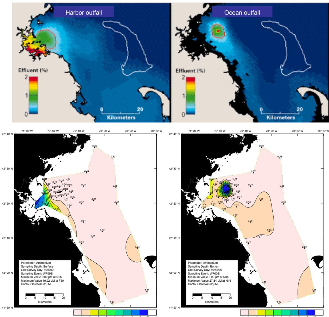
Figure 6-3. Model predictions for effluent dilutions from Deer Island (top left) and Massachusetts Bay (top right) outfalls; measured ammonia concentrations from pre-discharge and post-discharge, October 1999 (bottom left) and October 2000 (bottom right).
