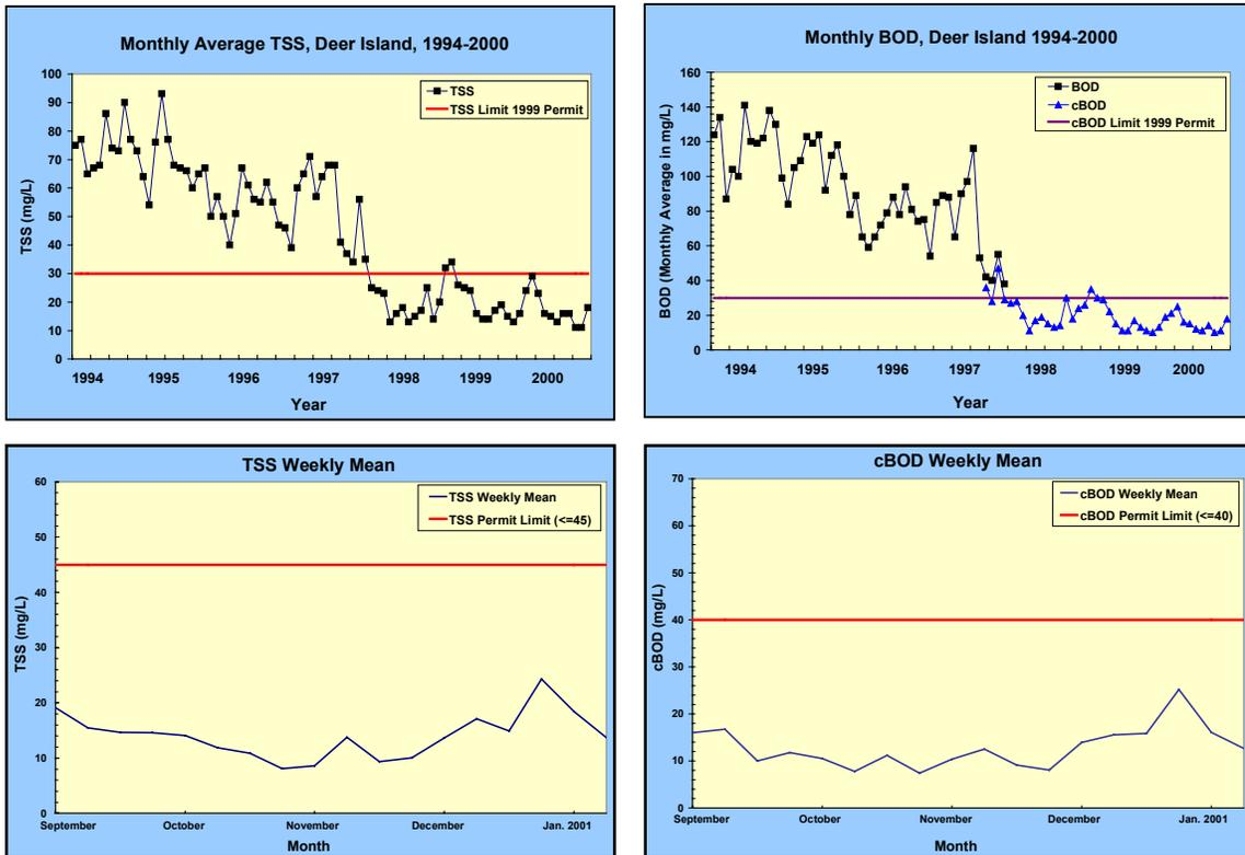
Figure 2-3. Monthly average TSS and monthly BOD (measured as cBOD since 1997) from 1994-2000. Weekly TSS and cBOD during the period in 2000 that the offshore outfall was discharging.
