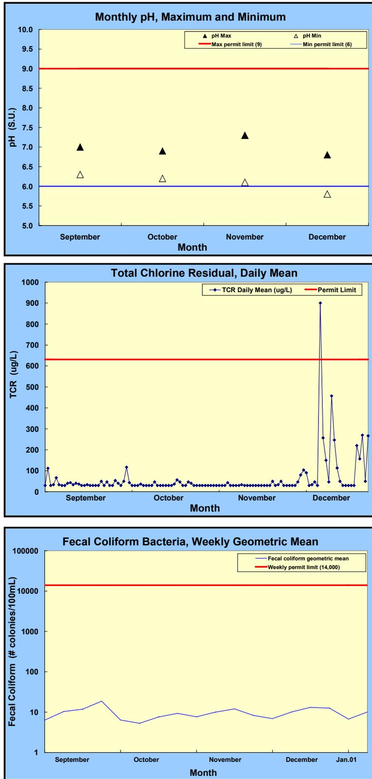
Figure 2-4. Monthly pH, daily mean chlorine residual, and fecal coliform bacteria data from the period in 2000 in which the outfall was discharging
