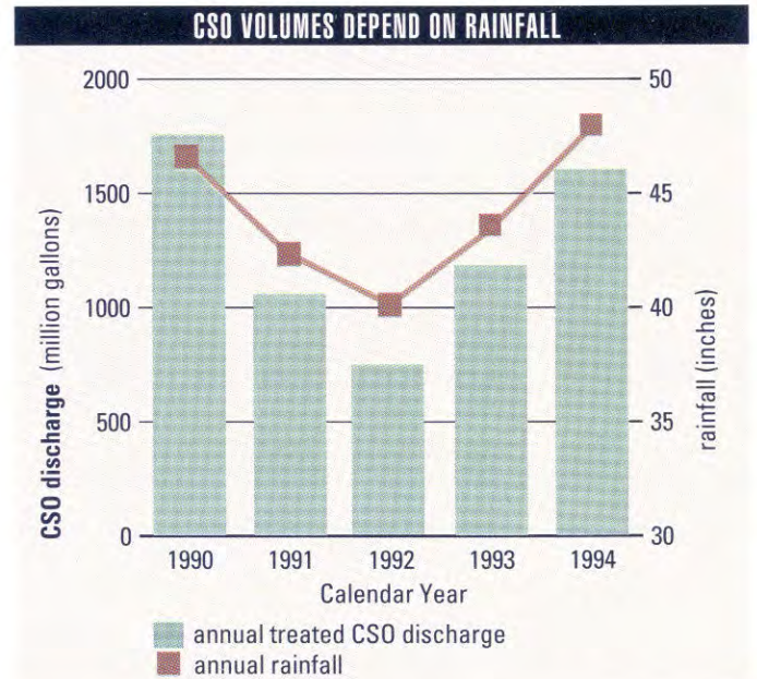
FIGURE 4: Combined sewer overflow volumes vary considerably depending on the number and size of storms. (Source: MWRA CSO treatment facility records)
