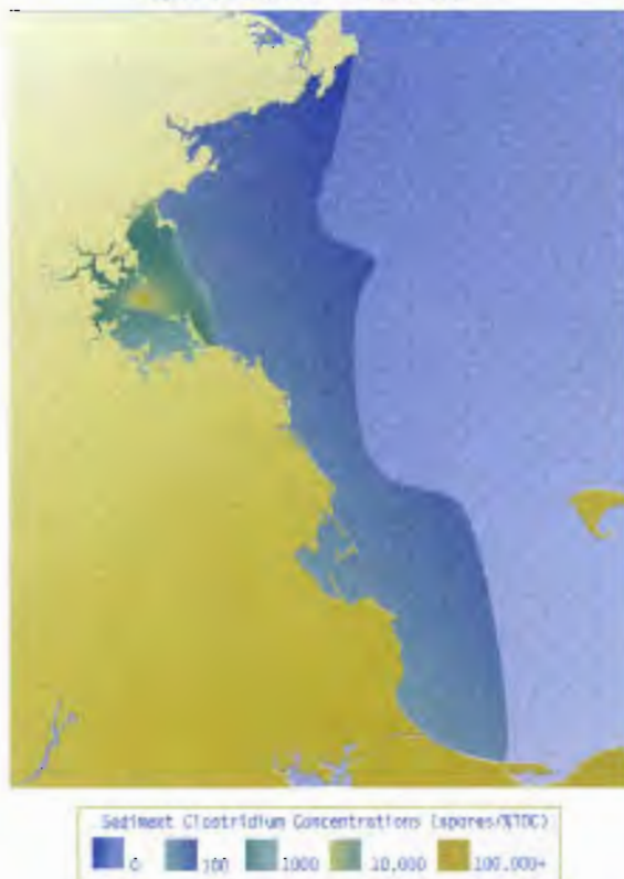
Distribution of sewage tracers documents the export of solids from Boston Harbor.
