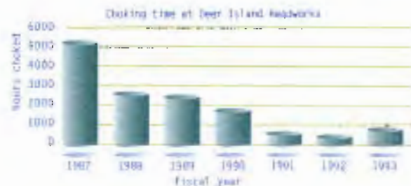
FIGURE 1.3. Total number of hours the headworks at Ward Street, Chelsea Dock and Columbus Park choked back flow between 1987 and 1993. A slight escape this year is primarily the result of construction related activity.
