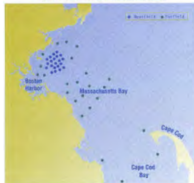
Figure 3.1 The MWRA's monitoring plan (one of the most sophisticated monitoring projects ever undertaken in the United States). Nearfield stations provide a detailed description of water quality in the area expected to be affected by the new outfall. Farfield stations monitor large scale trends across the bays and will identify any predicted impacts of the new outfall.
