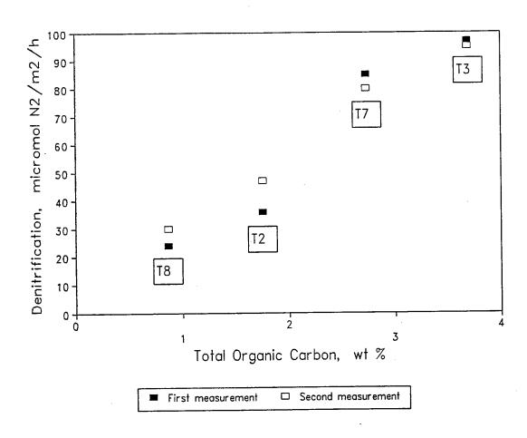
Figure 3: Relationship between Sediment Denitrification and Total Organic Carbon in Sediments.
